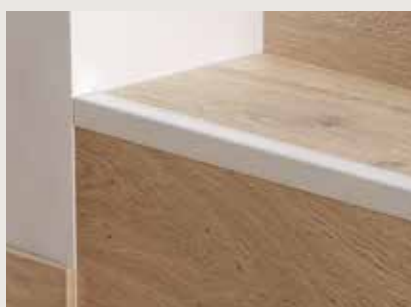
STAIR PROFILE SILVER 2500 × 50 × 25 mm. Fits flooring thickness 7 – 15 mm. Aluminium. PGSTPSILVME250
